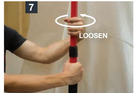
**7** When the job is finished, reduce height of pole by twisting counter-clockwise to loosen. Then unlock sheeting from head clip.
